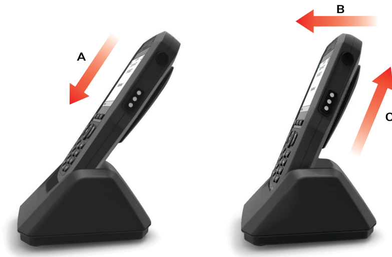
Figure 15. Example of how to insert and remove the handset from the desktop charger
