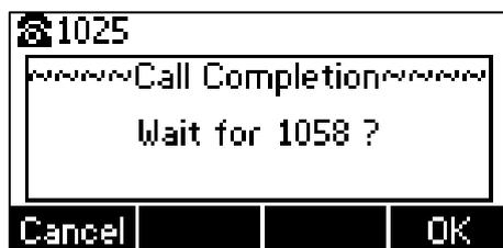
1. Press the **OK** soft key, the phone returns to the idle screen and call completion is activated.
