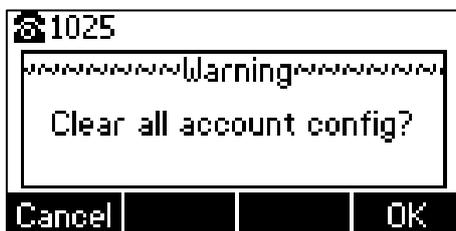
2. Press the **OK** soft key, registration configurations of all accounts on the phone will be cleared immediately.
