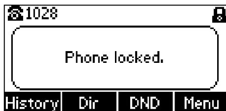
To unlock the phone, you must know the phone unlock PIN. The default phone unlock PIN is "123".
