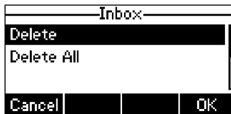
3. Select **Delete** to delete the desired message, then press the **OK** soft key. The LCD screen prompts "Delete message?".
