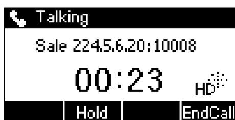
4. To place the current multicast RTP session on hold, press the **Hold** soft key.
