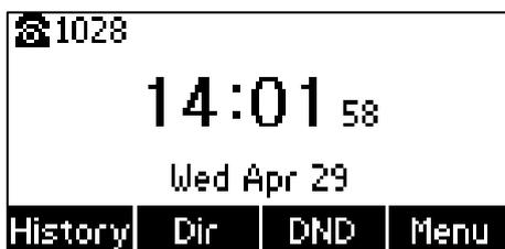
The idle screen displays the label of current account, time and date, and four soft keys.
