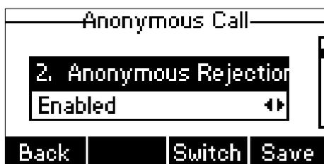
4. (Optional.) Press  $\leftarrow$  or  $\rightarrow$ , or the **Switch** soft key to select the desired value from the **Send Rejection Code** field.
